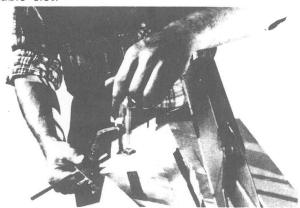
The Miter Gauge Stop Rod is used to cut several work pieces to the same length without repeated measurements. By adjusting the two steel rods, duplicate pieces may be cut to any length from 0" to 18". Two set screws are provided for locking the stop rod into either side of the MARK V miter gauge (on Shopsmith Model 10ER, see note below).
