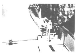
**Note:** The Miter Gauge Stop Rod can be used on either side of the miter gauge, depending upon whether the gauge is used in the right or left table slot.
